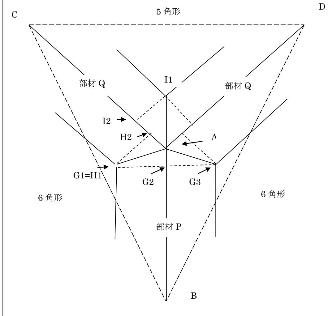
$$AB = AC = AD = \frac{3\sqrt{2}}{\sqrt{21-\sqrt{5}}} L \quad BC = DB = \sqrt{3}L \quad CD = \frac{\sqrt{5}+1}{2}L$$
